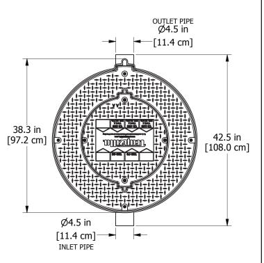
10 in [25.4 cm] CLEARANCE FROM TOP OF TANK REQUIRED FOR LID REMOVAL
