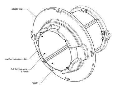
Step 6: Place the adapter ring/extension collar assembly onto the Trapzilla unit. Position the small cover onto the extension collar. Secure the adapter ring and the small cover with the brass nuts and flat washers provided. Seal the gap between the 18" extension collar and extension collar adapter ring using a silicone sealant.
