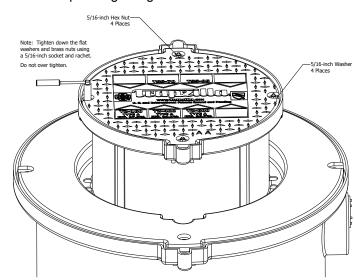
IMPORTANT: Excess extension collar must be trimmed on all units. Do not allow additional extension collar to extend beyond bottom of adapter ring. On units where extension collar is completely recessed, the extension collar should still be secured and the excess extension removed as in step 3.
