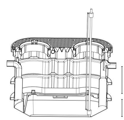
Take grease measurement from top of liquid level downward and compare to chart above.
