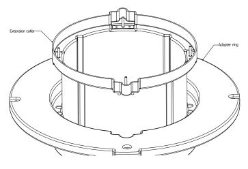
Step 5: Working from the bottom of the assembly, install eight (8) self-drilling, self-tapping screws (provided) through the extension collar wall and into the adapter ring. Two of these screws should be installed in each of the four (4) skirt areas of the adapter ring. Check the extension collar height dimension frequently during this operation to ensure that the collar has not moved. Note: Use caution when tightening these screws to ensure that they do not strip.
