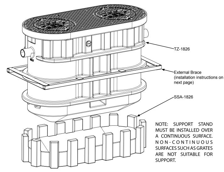
The SSA-1826 Support Stand is a one-piece assembly with a conical center that sits on the floor. It does not add appreciable height to the assembly.
