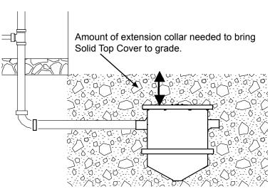
Step 1: With the Trapzilla unit installed in its permanent location, raise the telescoping extension collar to finished grade or floor level. Measure the height from the top of the unit to this finished extension collar height and record this dimension.
