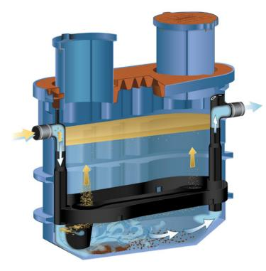
curve technology. This means that the unit does not lose grease separation efficiency as it fills with retained grease. Thus, the Trapzilla stores large quantities of grease without losing efficiency. The unique compact design of the Trapzilla allows for installation into most facilities. Options are available that enable a Trapzilla unit to be installed on the floor, suspended from the ceiling or in-ground outside the facility.
