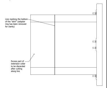
Step 4: Reinsert the extension collar into the adapter ring ensuring that the cover alignment key on the extension collar is aligned with its recess in the adapter ring. Reset the extension collar height to the dimension determined in Step 1.
