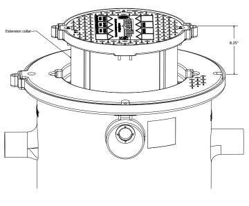
Step 2: Remove the extension collar adapter ring from the unit with the extension collar still in place. On the underside of the cover, mark the excess extension collar length at the bottom of the four (4) "skirt" portions of the adapter ring. Check the extension collar height dimension frequently during this marking to ensure that the collar has not moved. Extend this mark between the gaps in the "skirt" so that the collar is marked all around.
